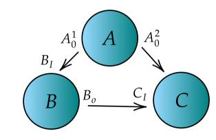
A DAG representing a quantum causal model. Two channels connecting the parties:  $T^{A_0^1 B_I}$  and  $T^{A_0^2 B_0 C_I}$
